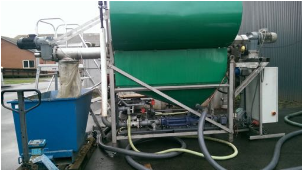
Figure 2. Photo of the PURROT® module during the test on site 2 (the biogas plant of Aarhus University). The solid output fraction is collected in the blue container to the left.
